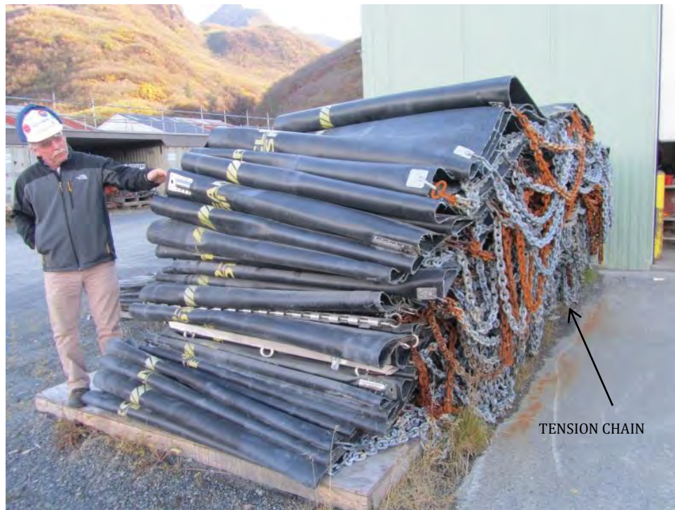
Figure 6. Deflated Ro-Boom 1500 (photo by M. Kartezhnikova)
