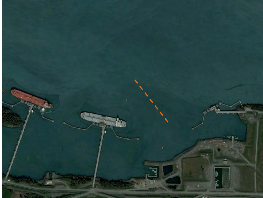
Figure 18. Possible floating breakwater location (dashed line)
